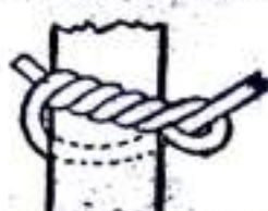
TIMBER HITCH for securing the end of a rope to a spar or log.
