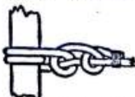
Round turn and TWO HALF HITCHES for tying a rope to a post.
